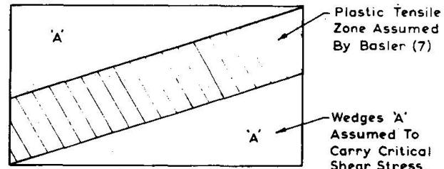
FIG. 3. COLLAPSE MODE ASSUMED
