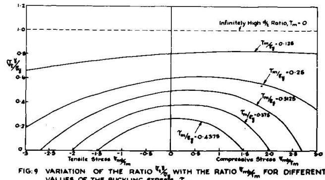
FIG. 9 VARIATION OF THE RATIO  $\frac{\sigma_t^Y}{\sigma_y}$  WITH THE RATIO  $\frac{T_m}{\sigma_f_m}$  FOR DIFFERENT VALUES OF THE BUCKLING STRESS  $T_m$ .
