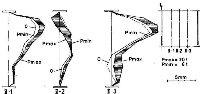
Fig. 18. Lateral Deflections of Web of Girder F-6.
