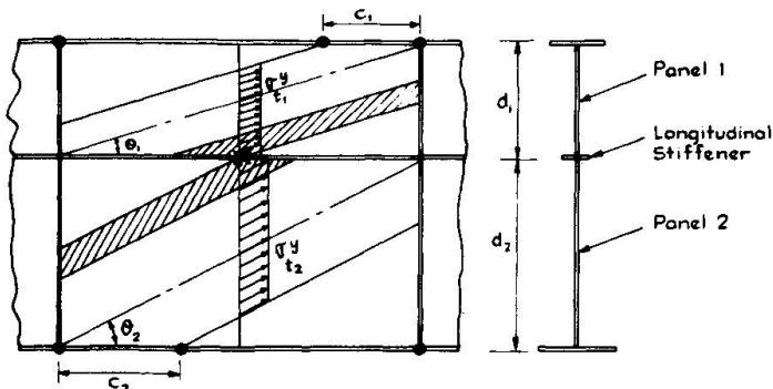
FIG.12 PROPOSED COLLAPSE MECHANISM FOR A LONGITUDINALLY REINFORCED WEB SUBJECTED TO SHEAR
