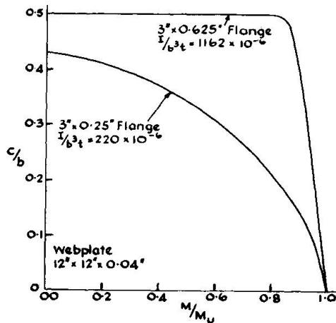
FIG.11 VARIATION OF THE  $\frac{c}{b}$  RATIO WITH THE MOMENT RATIO  $M/M_u$
