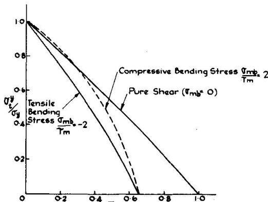
FIG. 8 VARIATION OF  $\frac{\sigma_t^Y}{\sigma_y}$  RATIO WITH  $\frac{T_m}{T_y}$  RATIO
