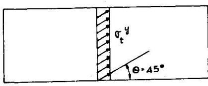
With very rigid flanges, such as occurs in an internal bay of a longitudinally stiffened girder, a normal tension field will develop and  $\theta \approx 45^\circ$
