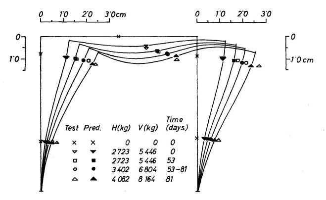
FIGURE. 4 Predicted and Test Deflection for Frame L1.
