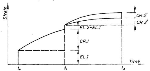
FIGURE 2(b) Total Strain Using Modified
