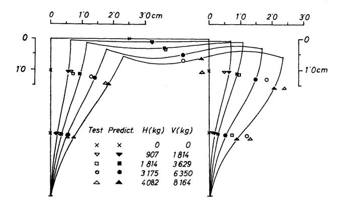
FIGURE 3 Predicted and Test Deflection for Frame R2.
