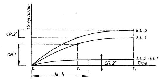
FIGURE 2(a) Creep Strain for Constant Stress.
