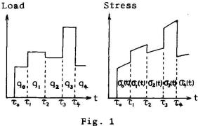
where  $E_c$  and  $\rho$  are modulus of elasticity and Poisson's ratio of concrete, respectively, and C(t,t) is creep function.
