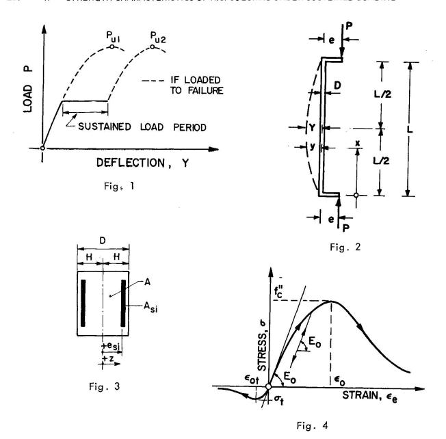
function',  $\theta$ . The adverse effects are taken a function of the stress intensity and the time over which the stress is maintained. Only stresses in excess of 70 per cent of the standard short time strength (at the time considered in the stress history) are assumed to have adverse effects on the strength. The strength variation model may be applied to any stress history, constant or variable.
