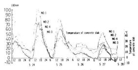
Fig. 6 Strain changes between girders. 24 ~ 28 MAY. 1968
