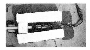
Photo. 3 Insulating case and differential transformer
