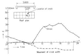
$\label{eq:Fig. 8} Fig. \ 8 \quad \text{Behavior on strain of bay between girders and} \\ \quad \text{width of crack}.$
