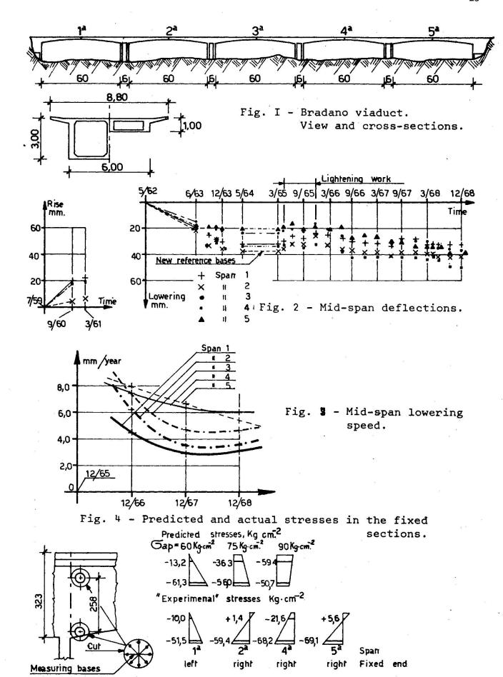
cutting into by core boring. The strains thus released have permitted to pass by means of Young's modulus  $\mathbf{E}_{\mathbf{b}}$  and Poisson's ratio
