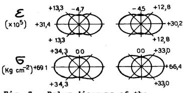
Fig. 7 - Polar diagrams of the strains and stresses released by core boring.
