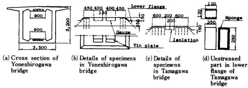
Fig. 4. Arrangement of concrete specimens for cut-out
