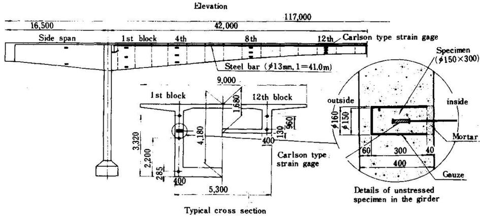
Fig. 1. Gage arrangement of Yagiyama highway bridge
