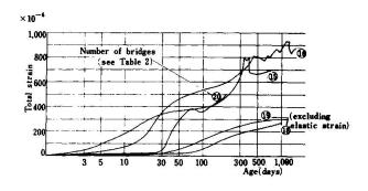
Fig. 7. Summary of measurements of delayed deformations in cantilever erected prestressed concrete bridges
