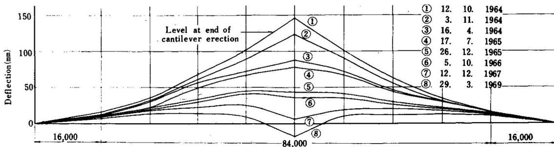
Fig. 3. Change of deflection at Yagiyama highway bridge
