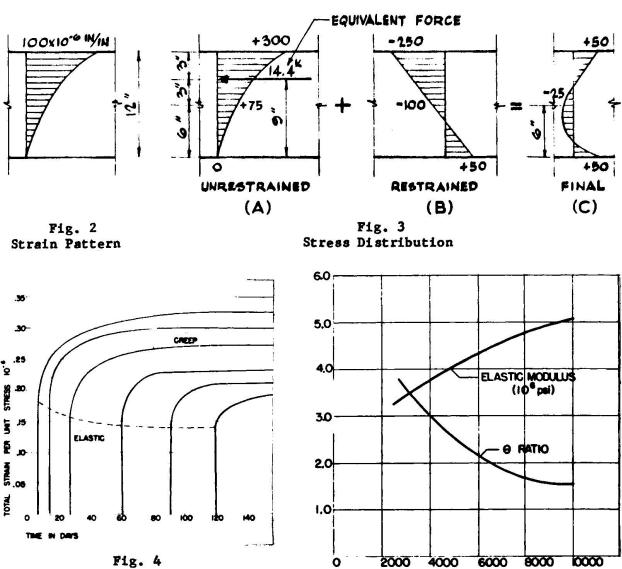
Total Strains Due to Constant Sustained Stresses Applied at Various Ages
