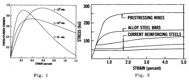
For high strength steels (alloy steel bars, pre-stressing wires) other equations consisting of an initial linear range and a subsequent non-linear range, can be introduced, without any change in the analysis.
