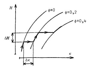
Fig. 8. Stepwise calculation of the additional time-dependent midpoint deflection.
