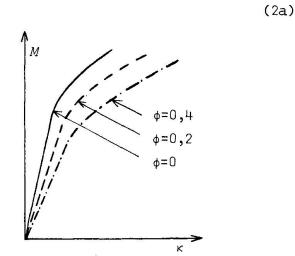
Fig. 7. Moment-curvature relationship for different loading times for a constant external normal force N.
