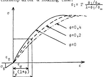
Fig. 6. Construction of stress-strain relationship for different loading times.
