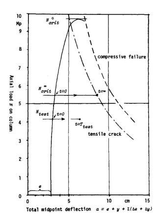
Fig. 10. Load-deflection diagram. Column A-2.
