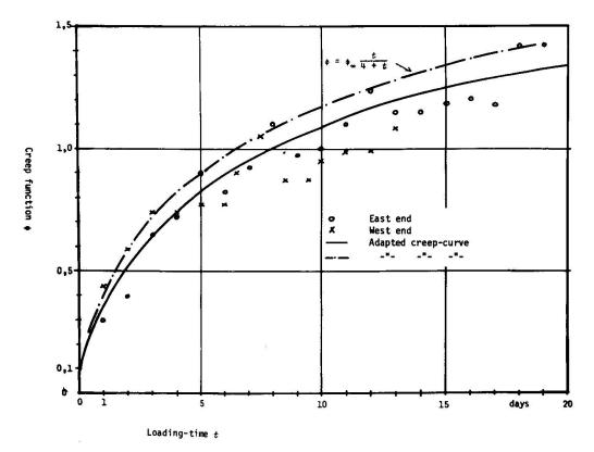
Fig. 4. Column A-2. Creep-function  $\phi$ .
