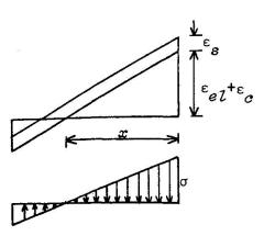
Fig. 3. Separation of shrinkage and creep. Evaluation of \$\phi\$ from measurements in the column ends.
