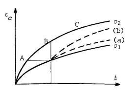
Fig. 5. A sudden increase of the stress level from  $\sigma_1$  to  $\sigma_2$  gives a strain increase following (a) when (3) is used. For concrete it would be more correct if the strain increase followed (b).
