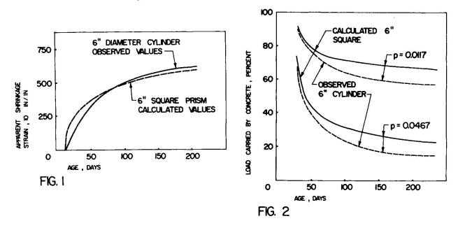
The effects of cracking were neglected in this study. Members subjected to axial compression may develop tension stresses due to shrinkage over a relatively small portion of the outer perifery of the cross-section. It is assumed that either these stresses are sufficiently small so that no cracking occurs, or if cracking occurs over a small area, then its overall effect is small.
