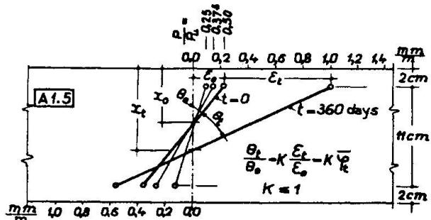
Fig.8. The rotation of cross section at mid span on loading and after 360 days (Beam A 1.5)
