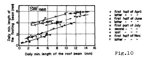
The figure clearly shows that there exists a linear relation between the two quantities for a period of one or two months and tnen suddenly another linear relationship appears. It would mean that some number of footings had a slip in the horizontal direction because of a too large change in length of the frame.
