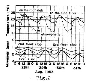
The observations on the movements of the expansion joint were started in August 1953 after a preliminary test for one month and were continued for about three years. The atmospheric temperature and the room temperature near the measuring apparatus were also recorded at the same time.
