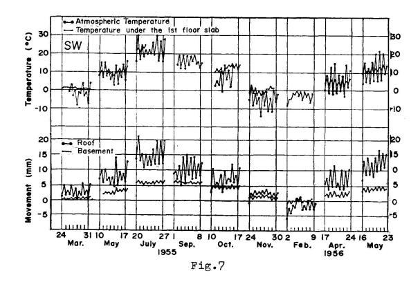
remarkable difference can be seen between the expansion in the south-west side frame and that of the north-east side frame. In this case, the north-east side frame showed the maximum expansion at 2 o'clock in the afternoon and then tended to contract, but the south-west side frame showed the maximum value about two hours later and the magnitude of expansion became more than twice of the former.
