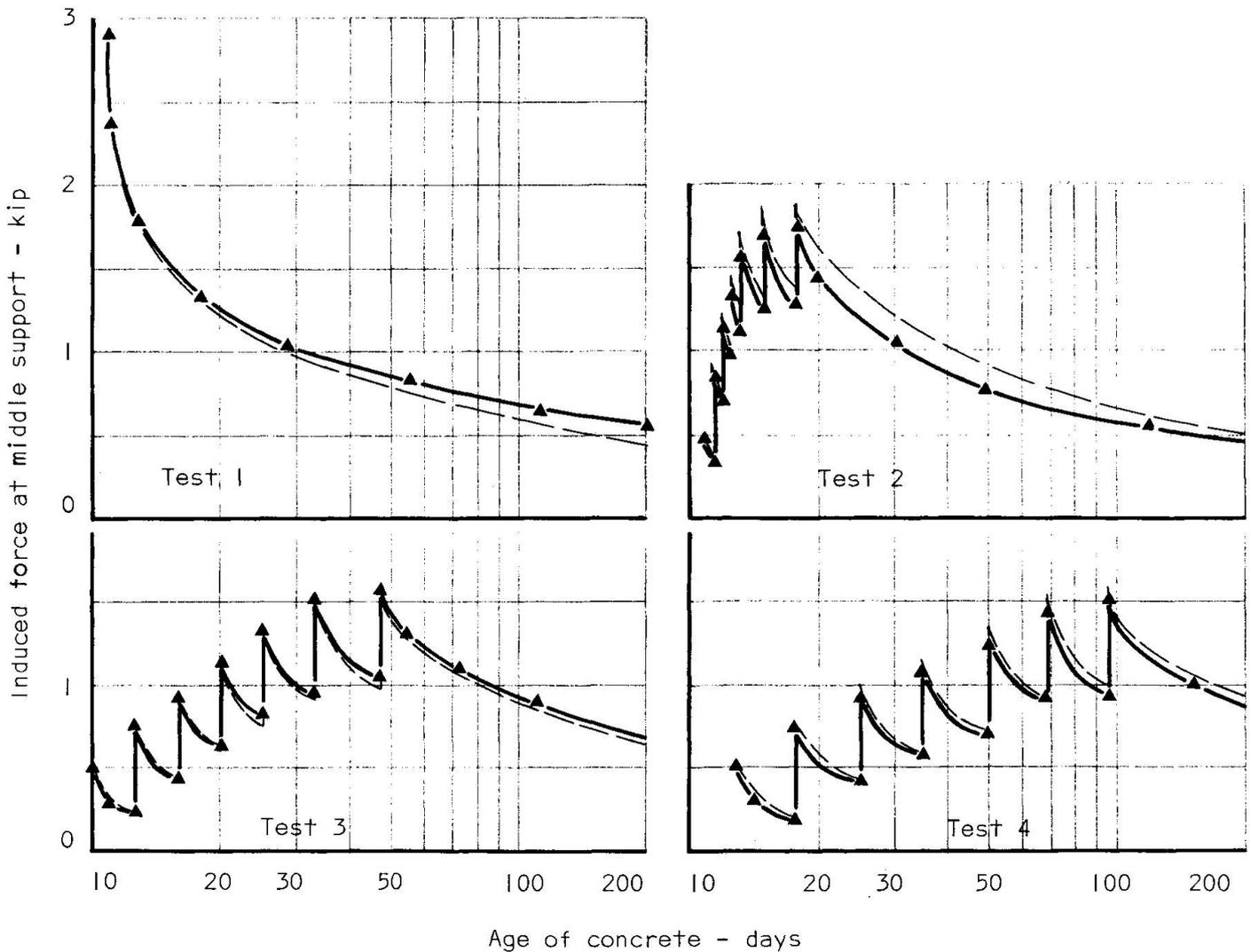
Fig. 5 Time-force relation for test beams
