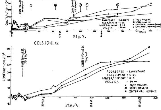
2 and 3 at 400 days, and 500 min\_columns 10 and 11 at 340 days, corresponding to steel stress of about 59.8 N/mm<sup>2</sup> and 96.5 N/mm<sup>2</sup> respectively. No attempt is made in this paper to evaluate the distribution of load between the concrete and steel in these columns.
