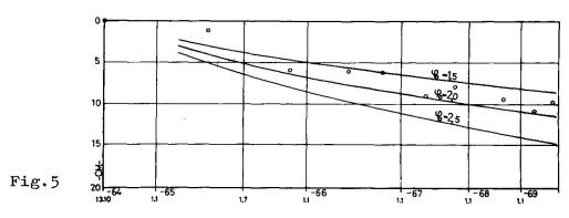
Fig.5 compares the results from the calculations and the observations of the 134 m midspan of the Alnö bridge. In this case a value of  $\phi_0$  of about 1.8 gives a satisfactory agreement.
