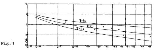
Fig.3 shows the results from the observations and calculations of the midspan of the Tunsta bridge. Its spans have the lengths of 41.1, 106.5 and 41.1 m. The observations form a rather irregular pattern but a value of  $\phi_0$ =2.0 gives a calculated deflection curve that on the average fits the observed values. Unfortunately no observations were taken during the years 1964-1968. The calculated deformations for  $\phi_0$ =1.5 and  $\phi_0$ =2.5 are shown as well.
