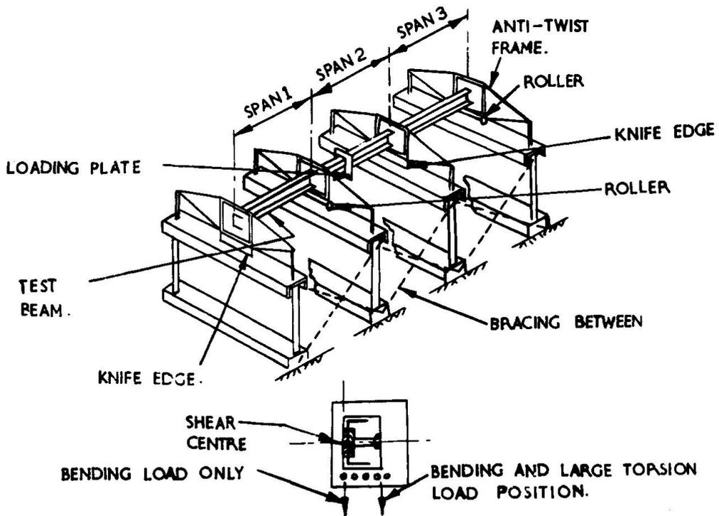
FIG. 1. DETAILS OF CONTINUOUS BEAM TEST RIG.
