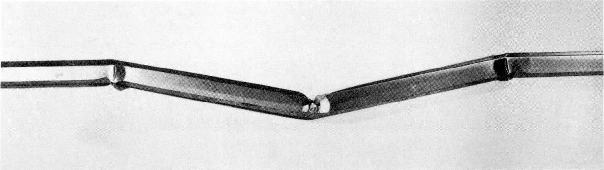
FIG. 4 (b) PURE BENDING COLLAPSE.
