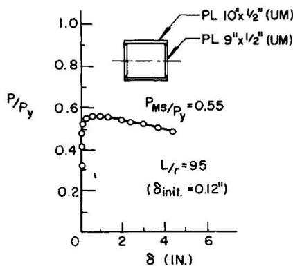
Fig. 1 Schematic load-deflection curves for simple columns
