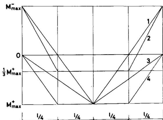
Fig. 7 - Moment gradients in test structures.
