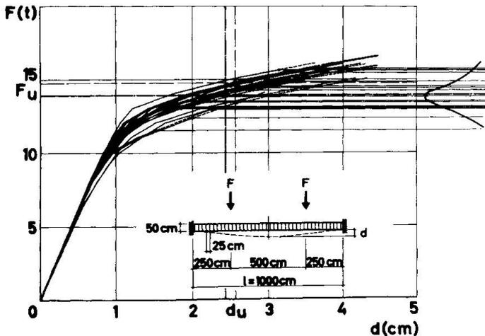
Fig. 4 — Load-deflection diagrams for structures 2.
