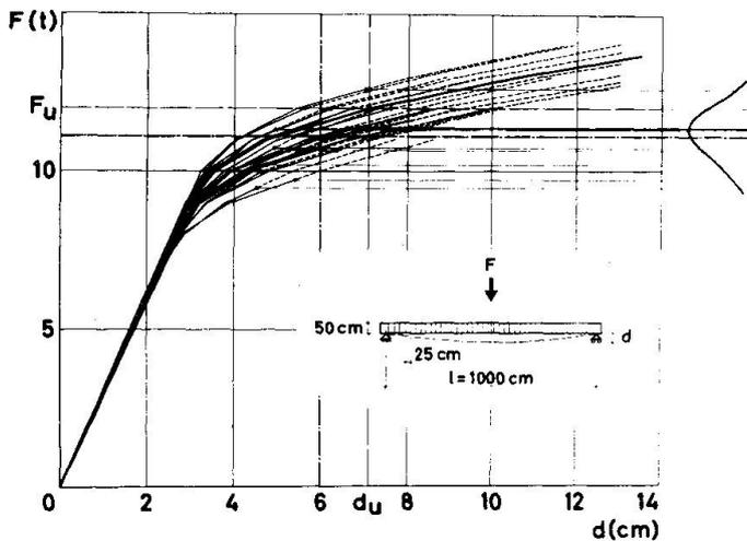
Fig. 5 - Load-deflection diagrams for structures 3.
