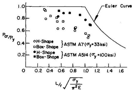
Fig. 11 Effect of yield strength on column strength
