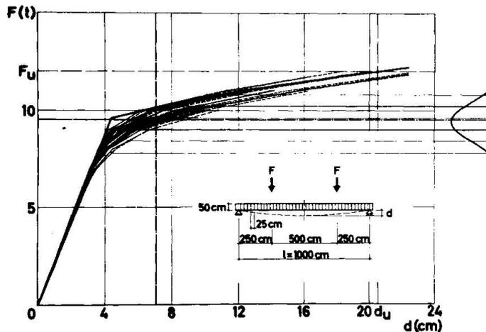
Fig. 6 - Load-deflection diagrams for structures 4.
