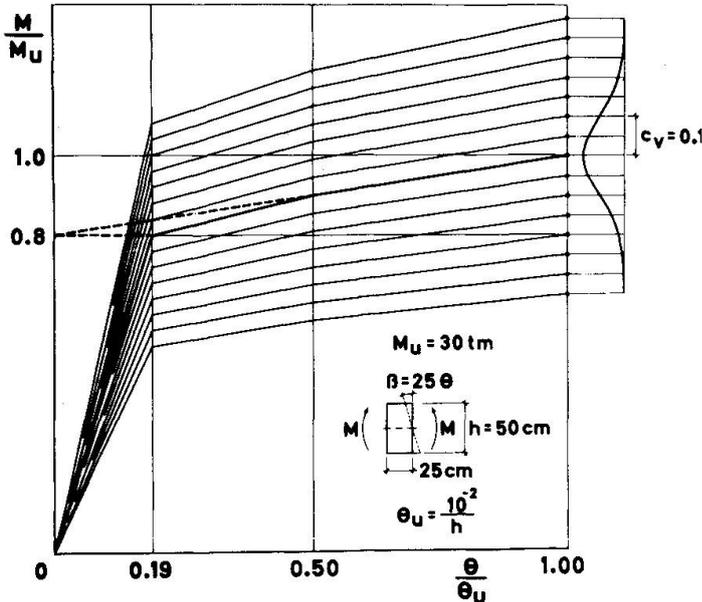
Fig. 2 — Trilinear moment-curvature diagrams.
