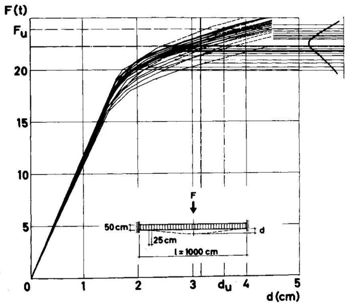
Fig. 3 — Load-deflection diagrams for structures 1.
