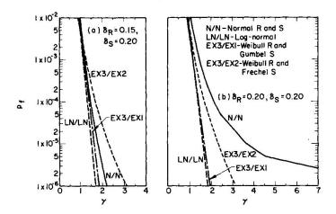
FIG. 1 SENSITIVITY OF 7 TO DISTRIBUTION FUNCTIONS (CLASSICAL RELIABILITY BASIS)
