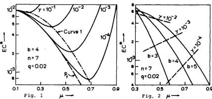
tivity of these items on the result will be an interesting subject of future study. For example, Fig. 2 shows the loci of the optimum points (such as Curve 1 in Fig. 1) for b=3, 4 and 5 plotted on the same diagram, indicating the effect of b and  $\gamma$  on the optimum proof-load.
