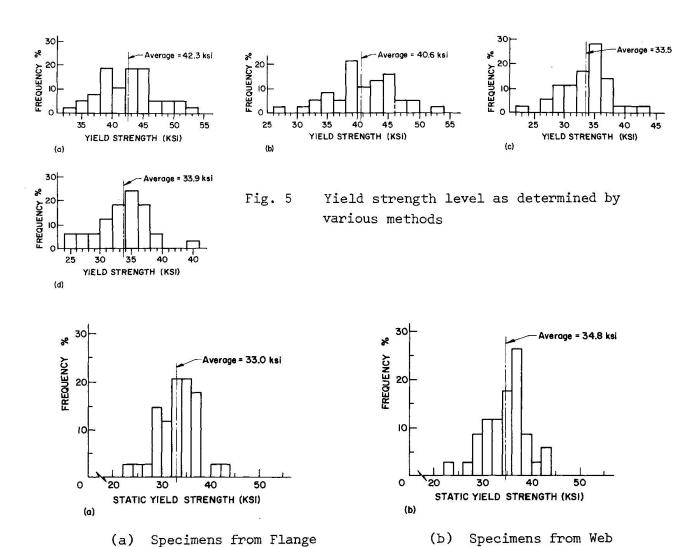
Fig. 6 Static yield strength of specimens cut from the flange and web of 34 H-shapes
