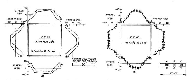
(a) Scatter between various fabricated lengths (b) Scatter within one fabricated length
