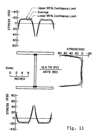
Residual stress distributions in three fabricated lengths of a welded H-shape 12H79. ASTM A572 (50) steel with nominal yield strength of 50 ksi
