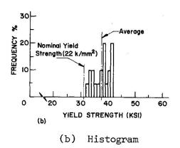
Variation of yield strength for specimens from various positions in the flange of an HE 200 B shape
