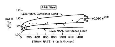
Fig. 4 Relationship between ratio of dynamic to static yield strength level and strain rate for ASTM A36, A441, and A514 steels
