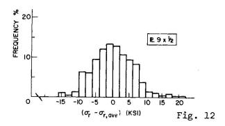
Histograms of residual stress results obtained from 10 different fabricated lengths of a welded box-shape 10 ☐ 65 (same results as in Fig. 10)
