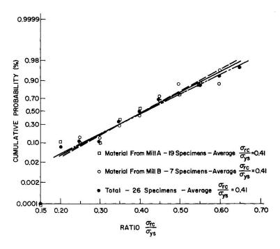
Fig. 13 Distribution of the ratio of maximum compressive residual stress to static yield strength for 26 hot-rolled wide-flange shapes
