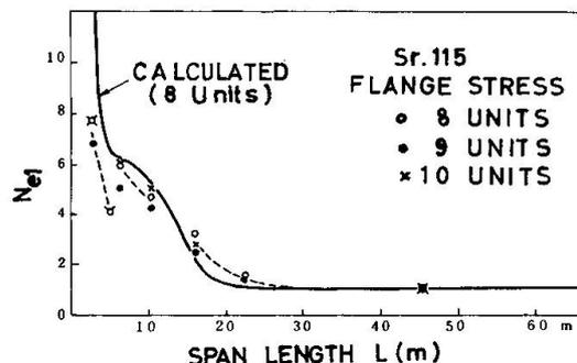
Fig. 7. L - N<sub>e1</sub> relation by electric railcar train (Series 115) measured on flanges of girder.
