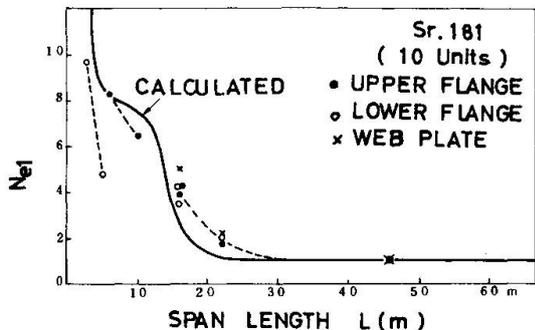
Fig. 6. L - N<sub>e1</sub> relation by electric railcar train (Series 181, 10 units).
