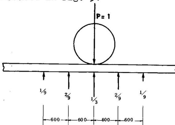
Fig. 4. Assumed distribution of load under sleepers.
