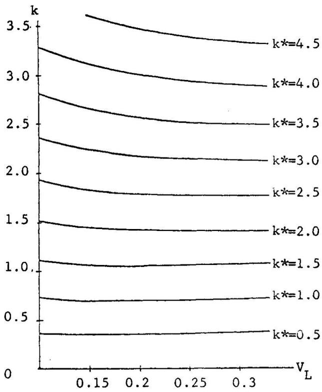
FIG. 4 CHART FOR DETERMINING RELIABILITY COEFFICIENT  $k - V_R = 0.15$
