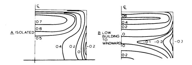
2. Pressure distribution on the windward face of a slab block (a) in isolation (b) with a low building to windward. (67.479.3)
