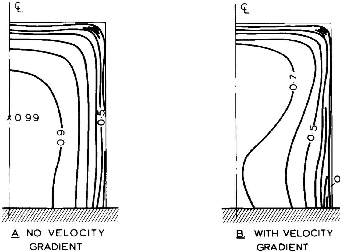
1. Comparison of  $C_{p_e}$  distribution on windward face of slab block in (a) uniform wind flow (b) flow with velocity gradient (67.479.4)
