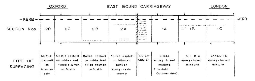
Fig. 2 LAY-OUT DIAGRAM. SEVERN BRIDGE TEST PANELS ON TRUNK ROAD A40 (WESTERN AVENUE), DENHAM, BUCKS, NOVEMBER 1963.
