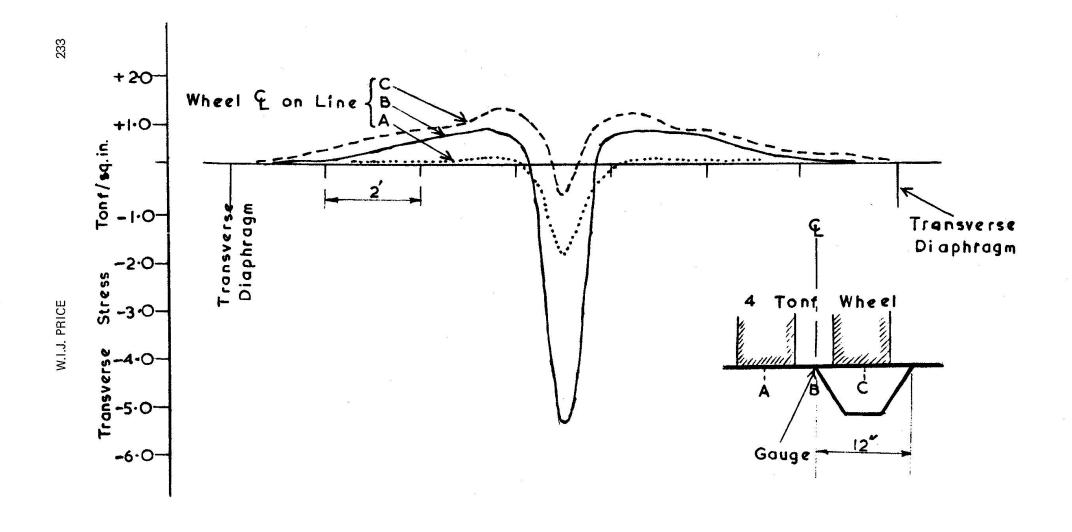
FIG. 8 TRANSVERSE STRESSES IN A DECK PANEL AT THE STIFFENER CONNECTION
