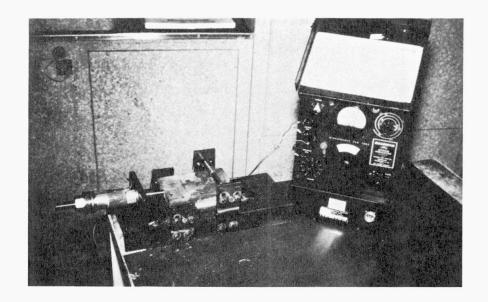
FIGURE 1. APPARATUS USED TO DETERMINE THE SHEAR BOND STRENGTH OF EXPERIMENTAL PAVING MATERIALS
