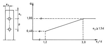
Figure 3.1. Factor  $\alpha$  as a function of the end distance.
