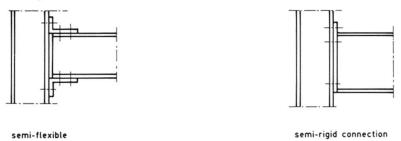
Figure 2.8. Semi rigid (semi flexible) connections.
