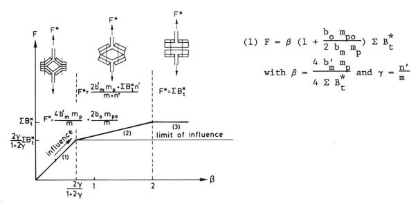
Figure 4.5. Effect of backing plates.
