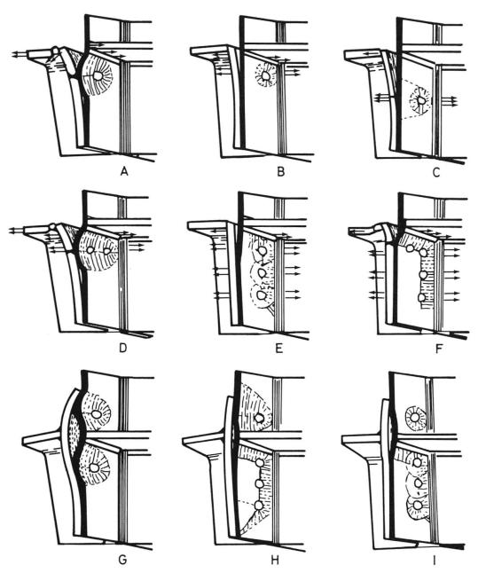
$\underline{\text{Figure 3.6}}$ . The effectiveness of added bolts depends on the yield line pattern formed by the first bolt.
