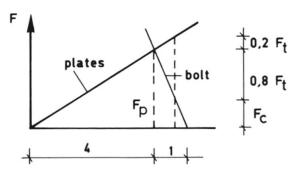
Figure 3.3. Load deformation curve of a preloaded bolt in a plate package.
