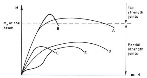
Figure 2.4. Moment-rotation curves of beam-to-column connections.
