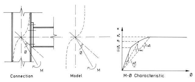
Figure 4.1. Modelling the connection by a rotational spring.
