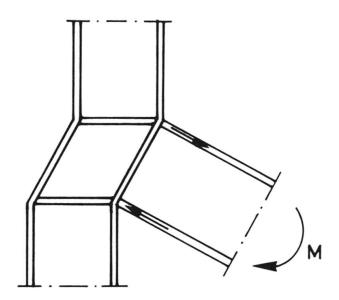
Figure 3.11. Shear panel failure.
