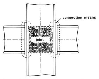
Figure 2.10. Beam-to-column connection.
