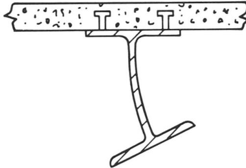
Fig. 2 Distortional lateral buckling of composite beam in hogging bending
