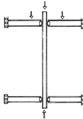
Fig. 5. Column sub-assembly
