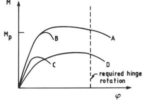
Fig. 9.  $M-\varphi$  curves for various connections
