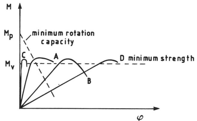
Fig. 10.  $M$ - $\varphi$  curves for unstiffened connections
