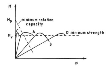
Fig. 10.  $M-\varphi$  curves for unstiffened connections
