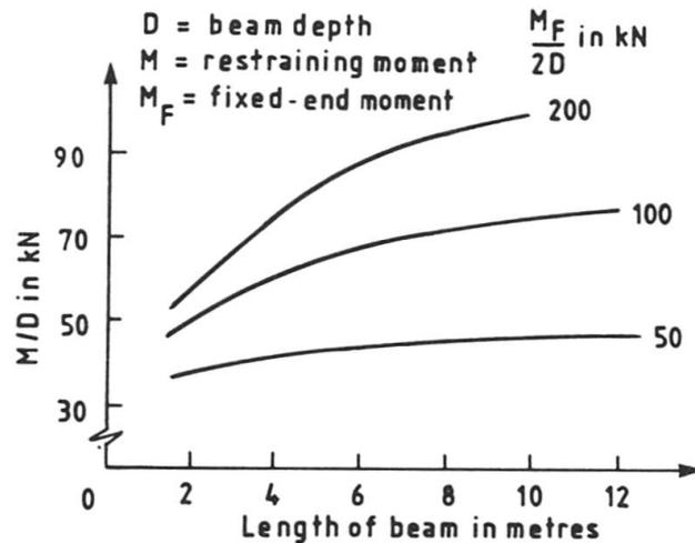
Fig. 8. Design using Class C connections [48]
