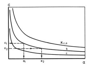
$\underline{\text{Fig. 4}}$  Stress vs. crack length for various  $K_{\underline{C}}$
