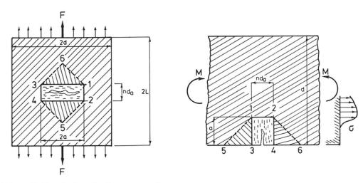
Fig. 7 Crack band; two examples
