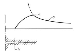
Fig. 6 Stress distribution in a fictitious crack
