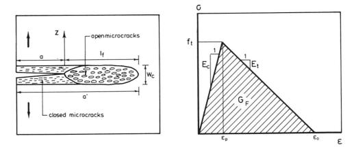
Fig. 8 Crack band and concrete schematization
