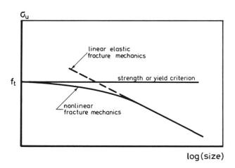
Fig. 9 Size effect according to various theories.
