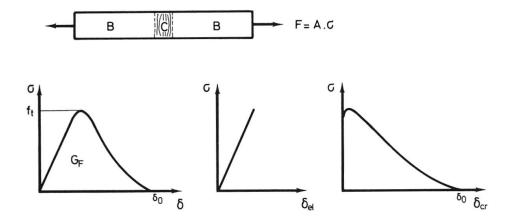
Fig. 5 Tensile specimen and stress extension curves
