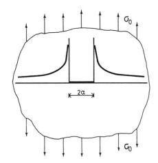
Fig. 2 Griffith crack
