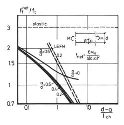
Fig. 13 Flexural strength of a cracked beam
