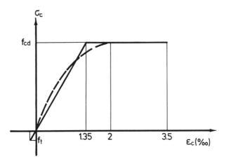
Fig. 1 Stress strain diagram of concrete
