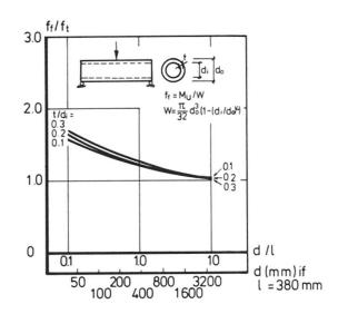
Fig. 14 Crushing strength of pipe as function of size
