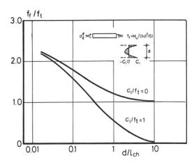
Fig. 12 Flexural strength with simultaneous shrinkage stresses
