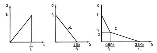
Fig. 10 Two examples of concrete modelling
