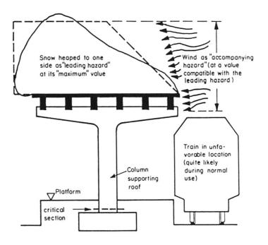
Fig. 2: Roof covering a platform of Railway station
