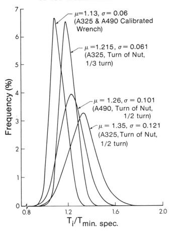
Fig. 9. Initial Bolt Preload for Various Installation Procedures
