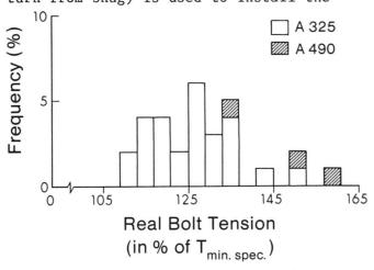
Fig. 8. Initial Bolt Preload: 1/3 Turnof-Nut Installation
