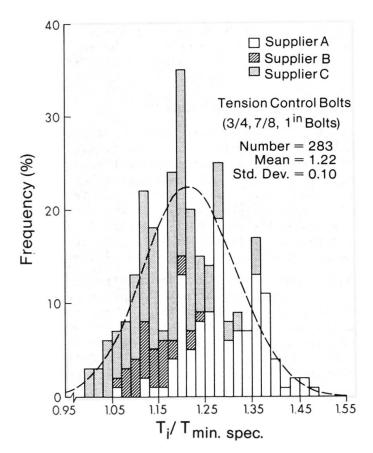
Fig. 10. Intial Bolt Preload for A325-Quality Tension-Control Bolts
