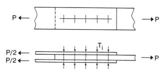
Fig. 1 Symmetric Shear Splice
