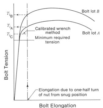
Fig. 5. Influence of Tightening Method on Bolt Preload
