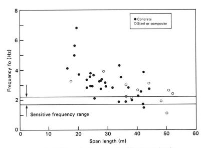
Fig.3 First bending frequencies for different span lengths
