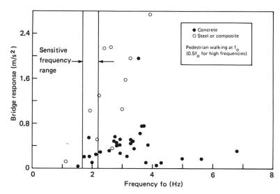
Fig.5 Bridge response to a pedestrian in relation to first bending frequency
