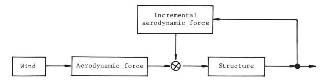
Fig. 1 Block diagram illustrating the onset of flutter
