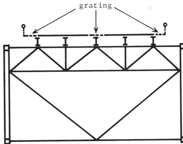
Fig. 10 Cross section of stiffening truss
