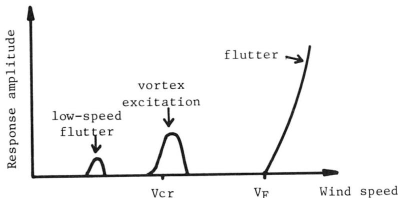
Fig. 2 Typical response of bluff structures in smooth wind
