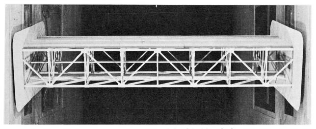
Fig. 14 Sectional model of bridge deck
