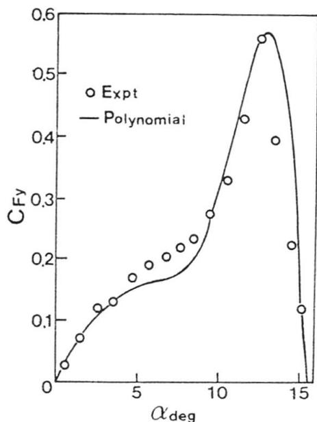
Fig. 4 Lateral force vs incidence for square prism [10]
