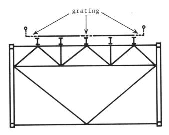
Fig. 10 Cross section of stiffening truss
