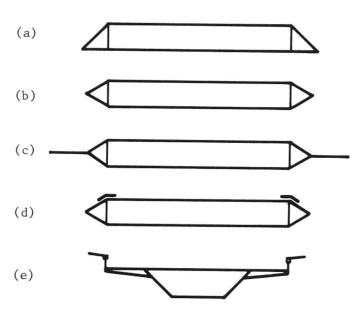
Fig. 11 Examples of stabilizers for bridge deck: (a,b) fairing, (c) fairing plus splitter plate, (d,e) flap
