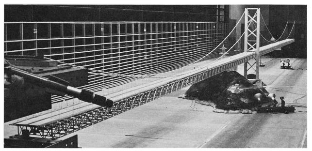
Fig. 12 Suspension bridge full model in wind tunnel
