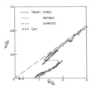
Fig. 5 Amplitude-velocity characteristics for galloping square prism [16]
