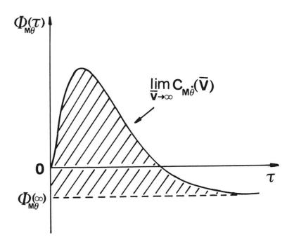
Fig. 6 Indicial aerodynamic moment response and the onset of torsional flutter
