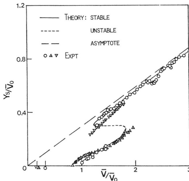
Fig. 5 Amplitude-velocity characteristics for galloping square prism [16]
