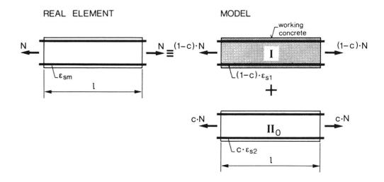
Fig. 1.2a Calculation model - pure tension
