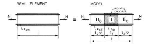
Fig. 1.2 Calculation model - pure tension
