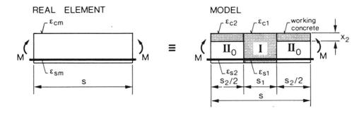
Fig. 1.3 Calculation model - pure bending
