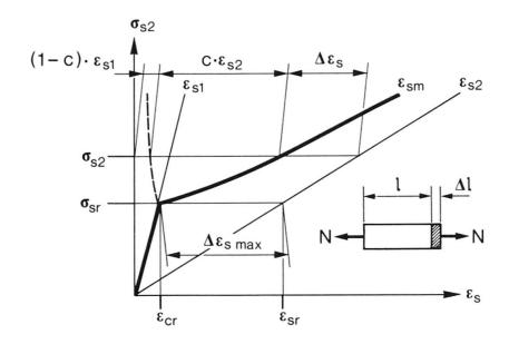
Fig. 1.1 Stress-strain curve for the reinforcing steel
