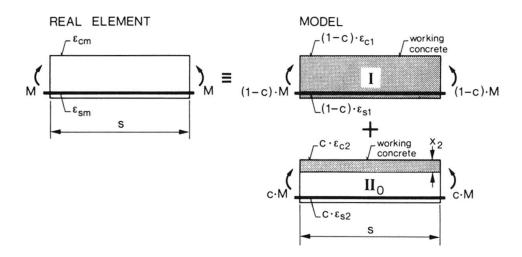
Fig. 1.3a Calculation model - pure bending
