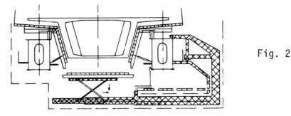
In both cases, the supporting structure itself is composed of either steel box girders or trusses. Formwork surface material is either steel or wood.
