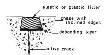
Fig. 3: Repair of Active Crack
