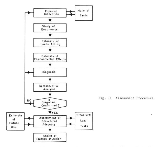
To minimise the likelihood of errors in assessment, a scientific, self-checking approach should be adopted. Such a procedure is shown in Fig 1 in the form of a flow diagram. In essence a tentative diagnosis is made on the available information, and is then confirmed (or rejected) by restrospective analysis of structural behaviour and, if appropriate, by re-inspection of the structure.
