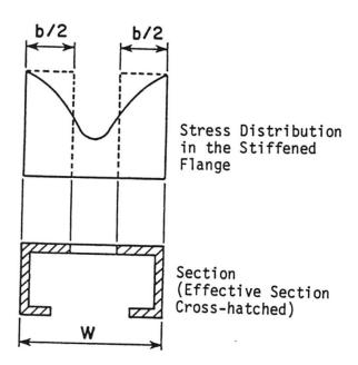
Fig. 10 Post Buckling Behavior
