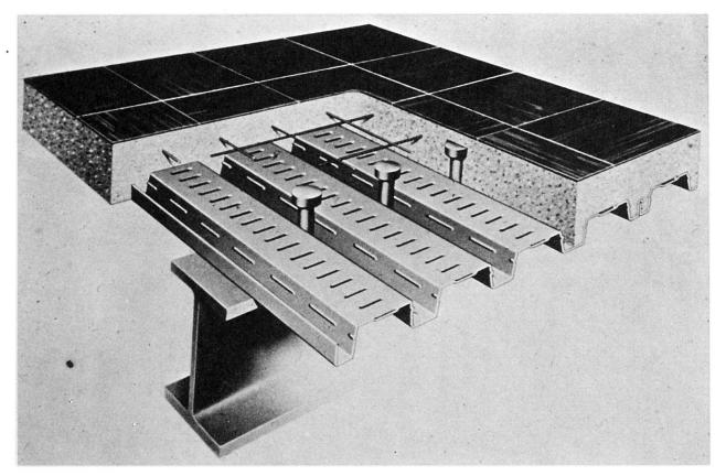
Composite Steel-Concrete in Both Fig. 4 Floor System:
