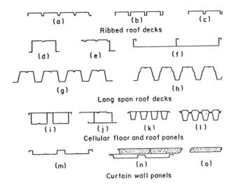
Fig. 2 Cold-Formed Steel Surface Members
