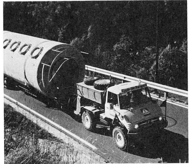
Fig.12 Transport of a FRP-silo (Constr.by Koloseus-Epple Wels, Austria)
