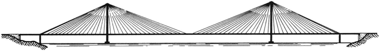
Fig. 4 Fan-shaped configuration of stay cables
