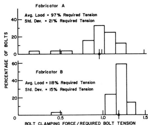
Fig. 4 Bolt Tension in 40 Bolt Truss Joints
