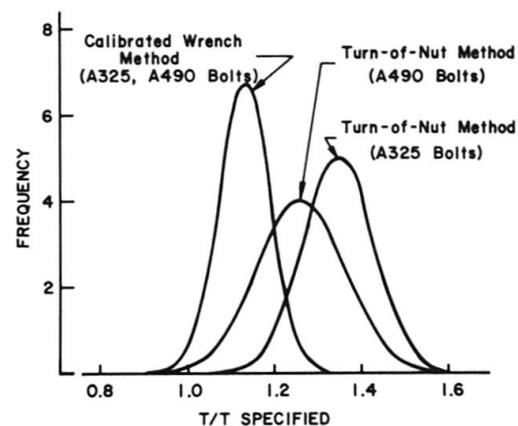
Fig. 3 Distribution Curves  $T/T_{\text{specified}}$  for Different Installation Procedures
