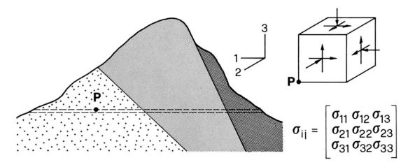
Fig. 2 Initial state of stress in the rock
