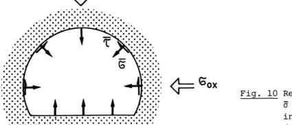
Fig. 10 Removal of boundary stresses  $\overline{\sigma}$  and  $\overline{\tau}$  according to the initial state of stress  $(\sigma_{OX}, \sigma_{OY})$
