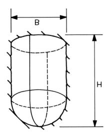
Fig. 3 Large underground chamber with statically favourable shape
