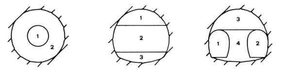
Fig. 5 Examples of multiple stage excavation in the tunnel section
