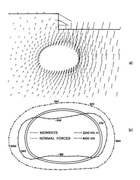
Fig. 17 Subway Munich: Computation No 15, (a) displacement field, (b) bending moments and normal forces
