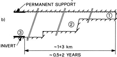
Fig. 6 Placement of an invert-arch
