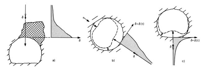
Fig. 20 Typical displacement fields associated with different types of rock pressure
