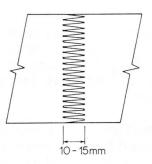
mini joints (for instance for individual laminations)
