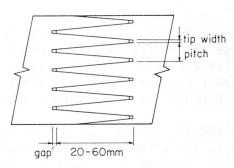
finger joints parallel to grain of laminated timber
