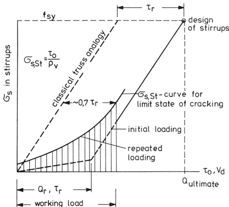
Fig. 14 Steel stresses in stirrups due to shear
