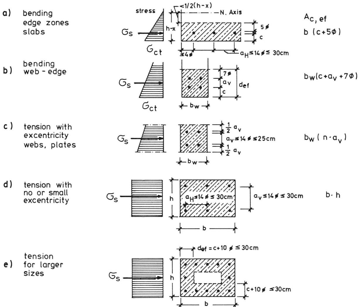
Fig. 8 Area  $A_{c,ef}$  around reinforcing bars, in which the bars enforce small crack spacing. For dimensioning crack spacing and crack width  $\rho_t$  must be related to  $A_{c,ef}$  and will be called  $\rho_{t,ef}$
