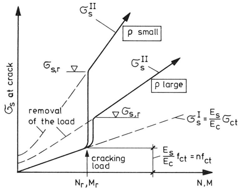
Fig. 3 Steel stresses in a crack of a prism under axial tension by increasing load for small and large  $\rho_t = \frac{A_s}{A_{ct}}$ .
