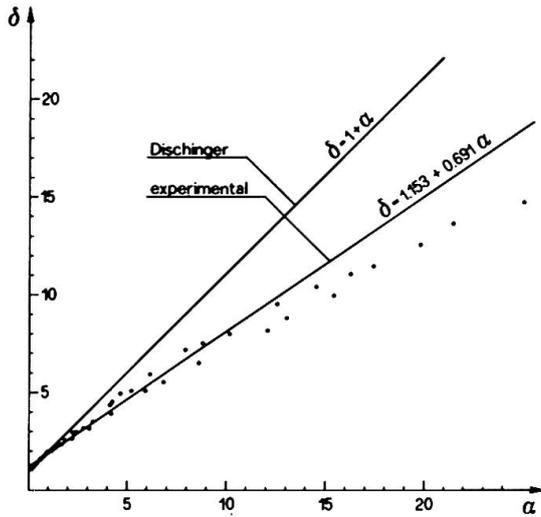
Fig. 18. Linear regression on  $\alpha - \delta$  data.
