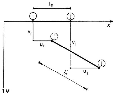
Fig. 4. Second model: finite element scheme.
