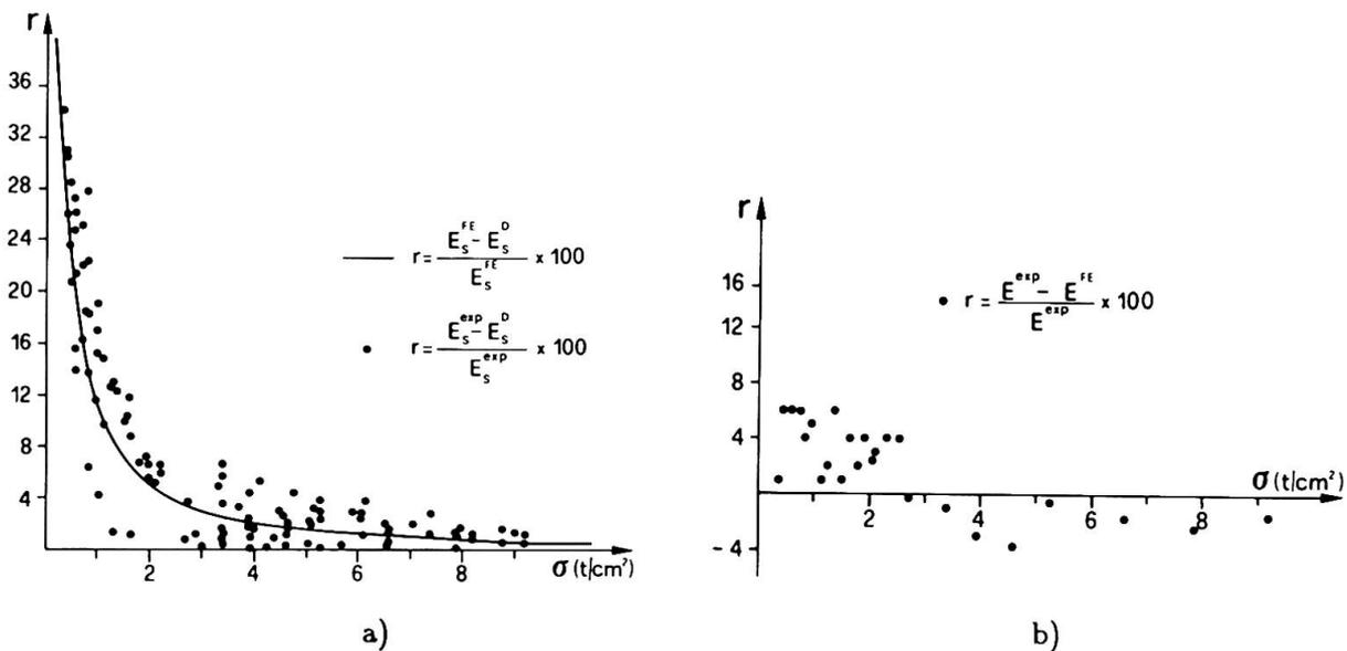
Fig. 17. Difference between theoretical and experimental values of the secant modulus versus stress levels.
