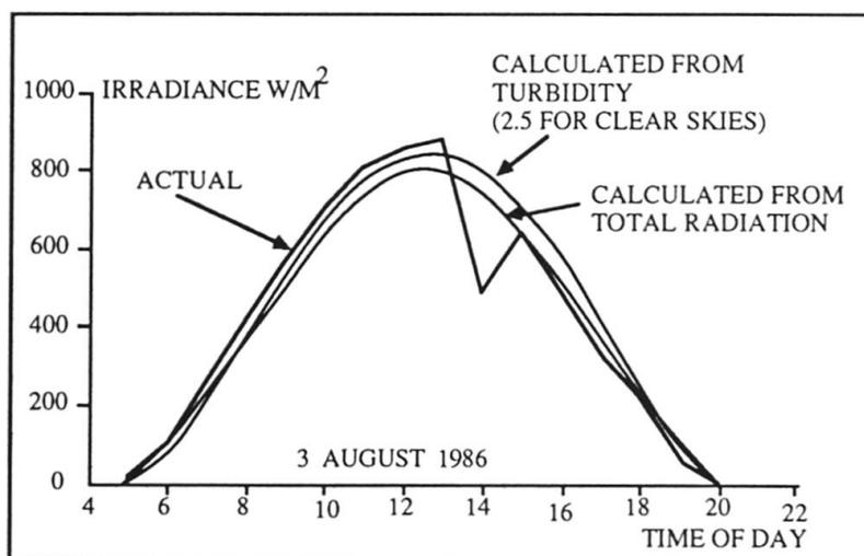
Fig. 3 Variation of irradiance, Calgary LRT Bridge
