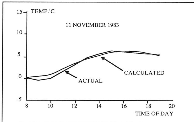
Fig. 12 Slab to girder differential, Cottonbush Creek.
