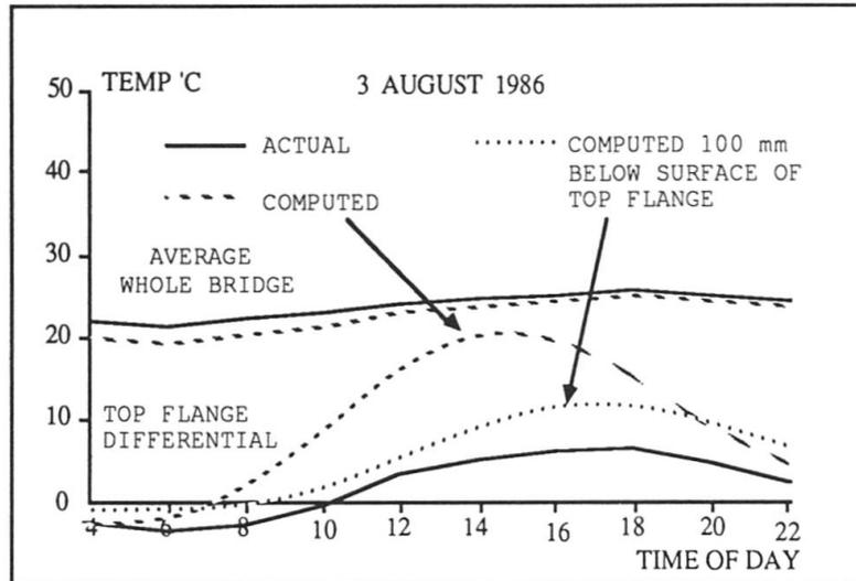
Fig. 6 Variation of temperatures, Calgary LRT bridge
