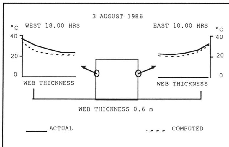
Fig. 5 Web temperature profiles, Calgary LRT Bridge
