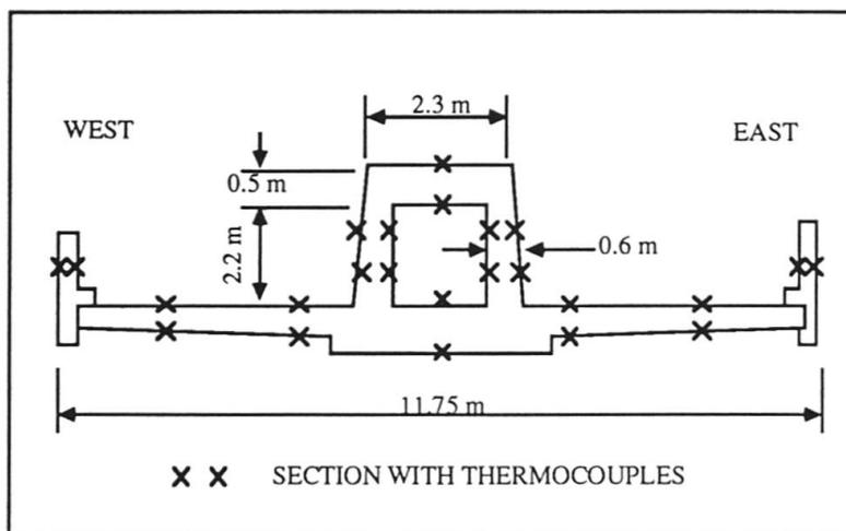
Fig. 2 Cross-section of Calgary LRT Bridge
