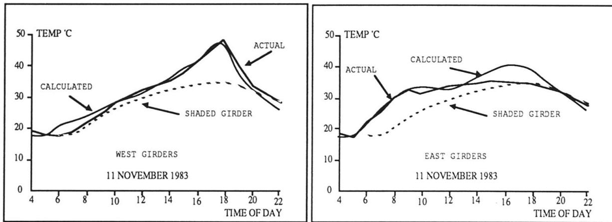
Fig 11 Variation of girder temperatures, Cottonbush Creek
