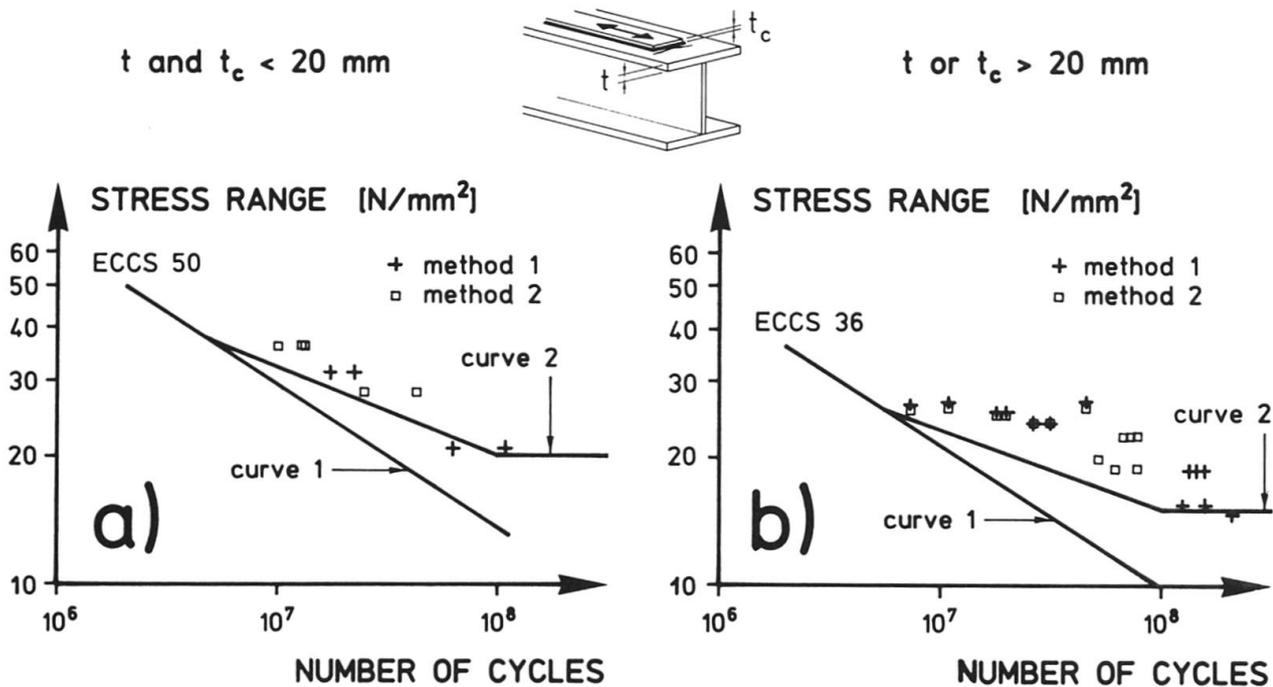
Figure 6. Variable-amplitude fatigue failures of coverplated beams [9-10].
