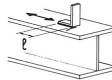
Figure 8. Variable-amplitude fatigue failures of beams with longitudinal attachments, 80 mm long [4].
