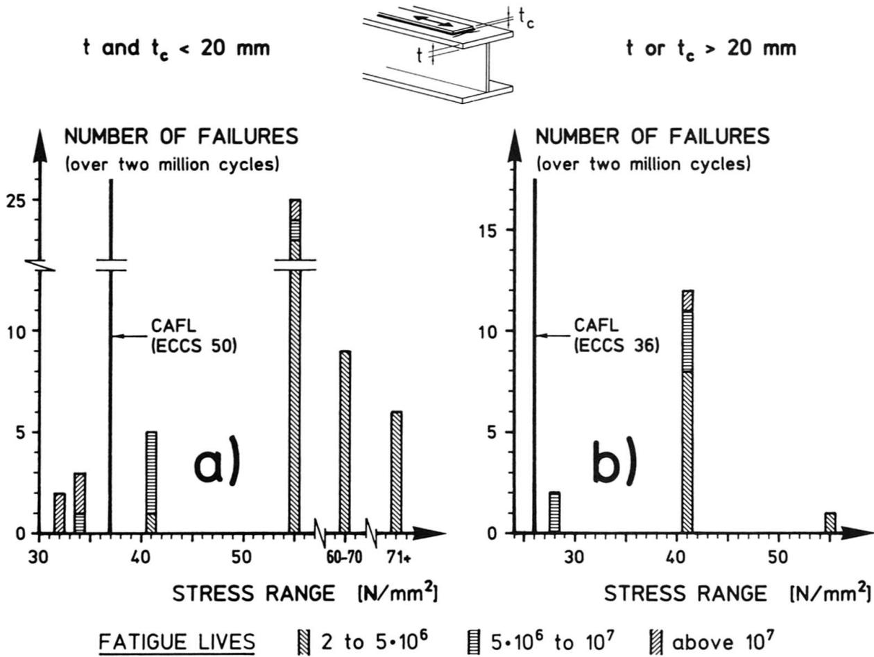
Figure 4. Constant-amplitude fatigue failures of coverplated beams [9] [16-20].
