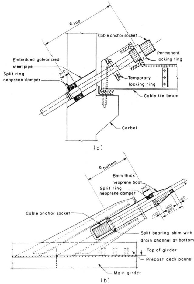
Fig. 2 Cable End Socket Detail Showing Split Neoprene Ring
