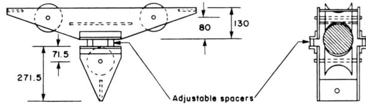
Fig. 6 Three-Wheeled Sensor Cart Used for Cable Tests
