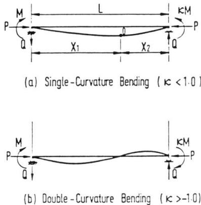
Fig. 6 Simply-supported columns
