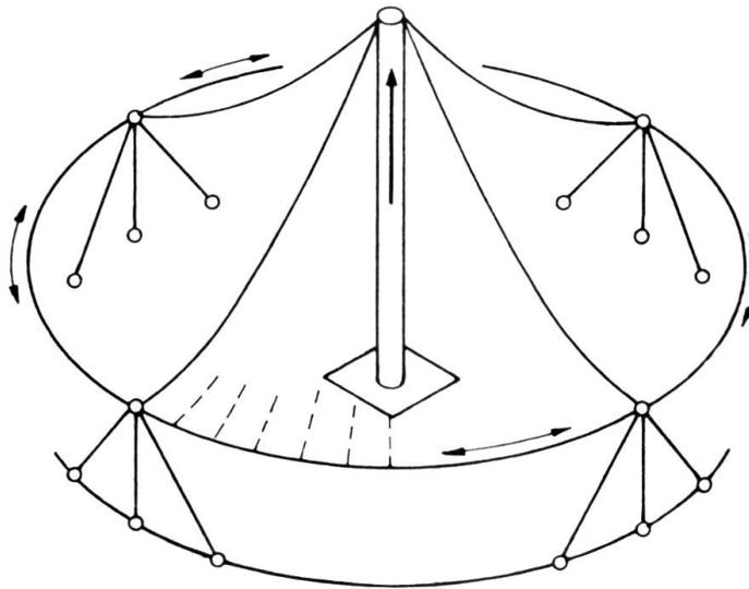
Fig. 4 : Structure with a lower circular ring. (No horizontal loading of foundation).
