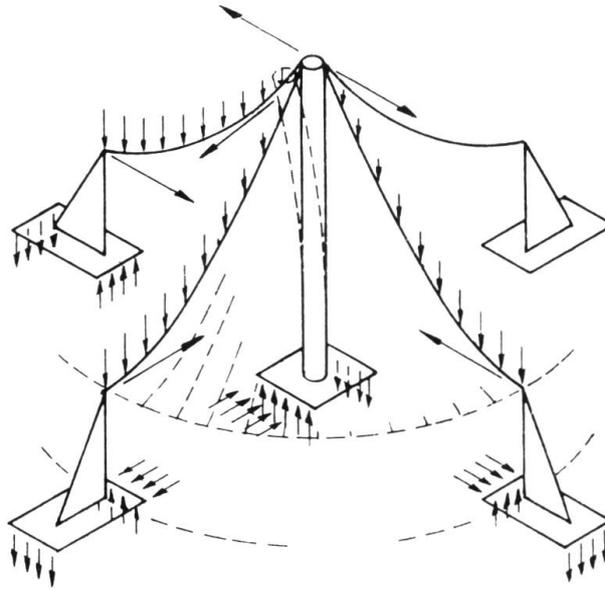
Fig. 5 : Structure with the suspension ribs a achored to each foundation
