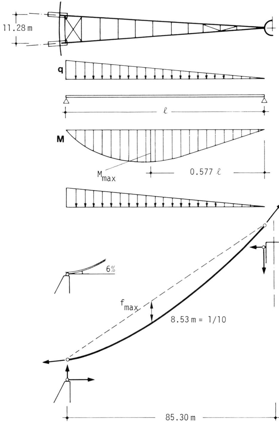
Fig. 3 : Determination of the shape of the ribs
