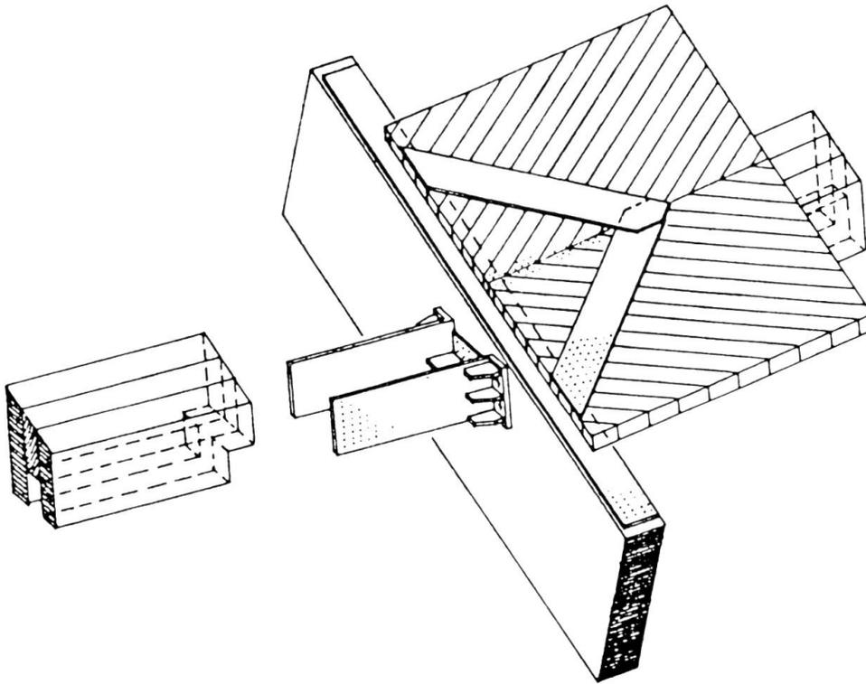
Fig. 11 : Connection between ribs, rings and boards.
