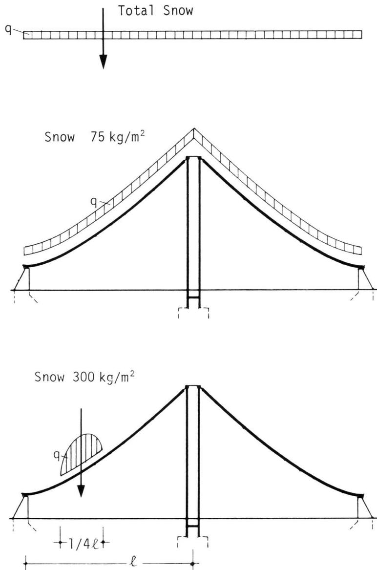
Fig. 8 : Calculated load case snow
